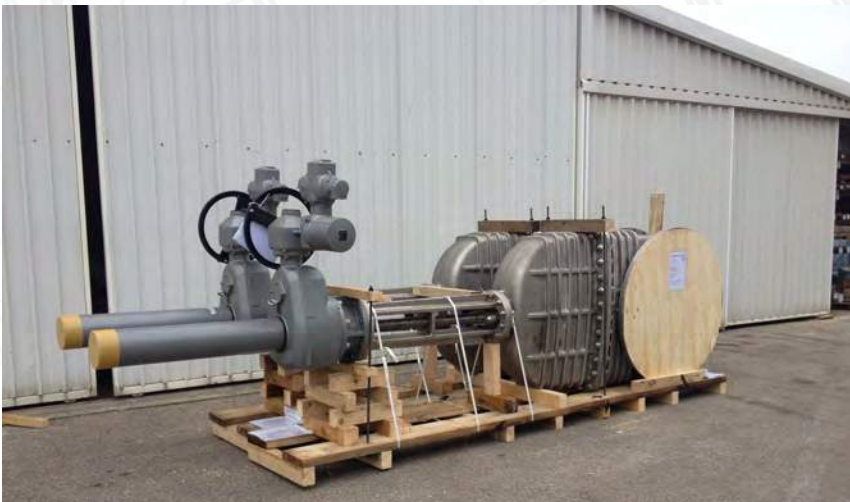
GATE VALVE DN 1000
