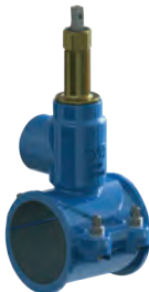
Series 727/09 Tapping saddle SWIC for underpressure drilling With integrated cutter for PE and PVC pipes DN50-200 Ductile iron
