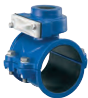
Series 727/10 Tapping saddle with blade shut-off For PE and PVC pipes DN80-200 Ductile iron
