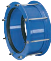
Series 258 Fabricated dedicated straight coupling for AC, steel, cast iron or ductile iron pipes DN350-2000 PN8 to 25 Steel
