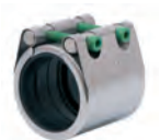
Series 745/20 Repico® slip coupling Universal and non-tensile for all pipes NBR or EPDM sealing DN15-600 Stainless steel AISI 316
