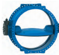
Series 756/102 Butterfly valve Double eccentric Double flanged Stainless steel seat ISO-input gearbox DN150-2800 PN10/16 Ductile iron
