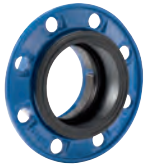
Series 05 Combi-flange for PE and PVC pipes Non-tensile (PVC) DN50-600 Tensile DN50-300 PN10/16 Ductile iron
