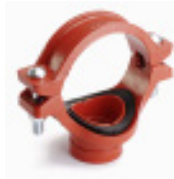
Series 230/86 Grooved mechanical Tee DN50-200 20,6 bar (300 PSI) Ductile iron UL/ULC listed, FM approved
