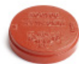
Series 230/75 Cap DN25-200 20,6 bar (300 PSI) Ductile iron UL/ULC listed, FM approved
