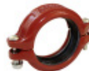
Series 230/04 Grooved coupling Flexible DN25-300 20,6 bar (300 PSI) Ductile iron
